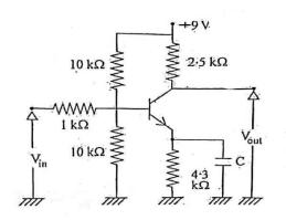
An amplifier in common-emitter configuration is shown in the above figure.
